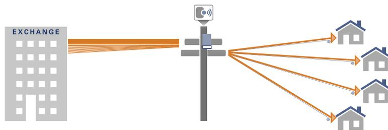
FIGURE 2B shows that the spare copper can be bonded to provide small cell backhaul.
