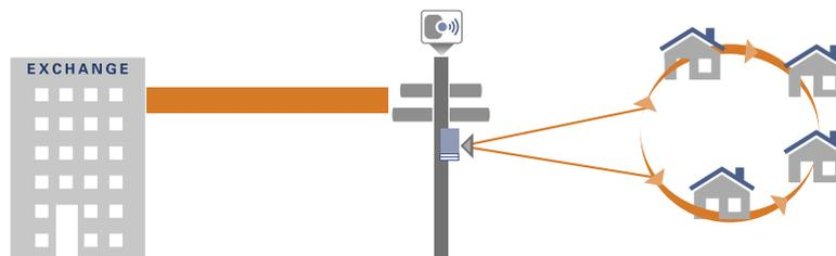
FIGURE 2C shows that by implementing the DSL Rings solution it is possible to share all aggregate bandwidth for the small cell service and fixed broadband to the home enabling maximum possible bandwidth to be delivered to both fixed and mobile users.
