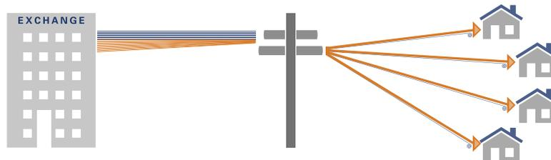
FIGURE 2A shows that not all copper pairs from the home to the distribution point are used and that there is spare capacity in the backhaul network.
